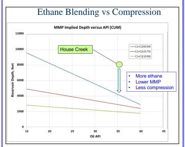
The blue arrow on the plot again shows that lower compression and flood pressure requirements require a higher percentage of Ethane to achieve miscibility of the enriched injectant.
